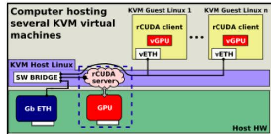
all the VMs. Two configurations are possible. In the first one (figure on the left) the GPU is located in the same host executing the VMs. In this case the virtual network provided by the hypervisor is used to communicate the rCUDA client and server. In the second scenario (figure on the right), an InfiniBand network fabric is available in the cluster. In this case, the rCUDA server can be placed in another computer in the cluster.
